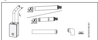
Fig. 20 Horizontal flue option
