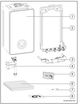
Fig. 1 Scope of delivery
