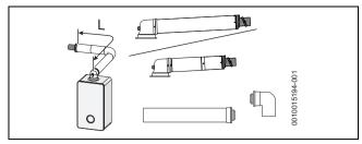
Fig. 18 Horizontal flue option
