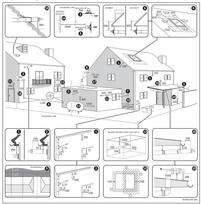
Fig. 31 Horizontal flue terminal positions
