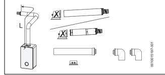
Fig. 21 Horizontal flue option
