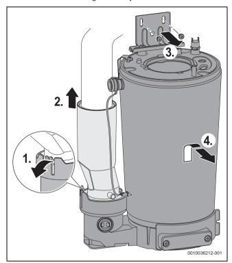
Fig. 86 Removing the heat exchanger assembly
