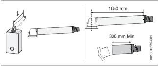
Fig. 16 Horizontal flue option
