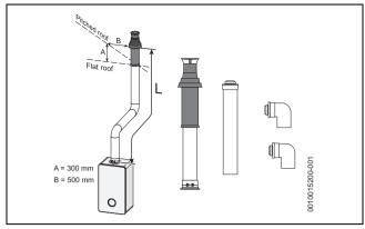
Fig. 25 Vertical flue option
