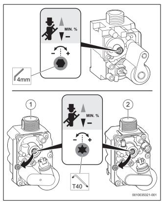
Fig. 82 Setting the CO<sub>2</sub> content (above: SIT valve, below: Honeywell valves)
