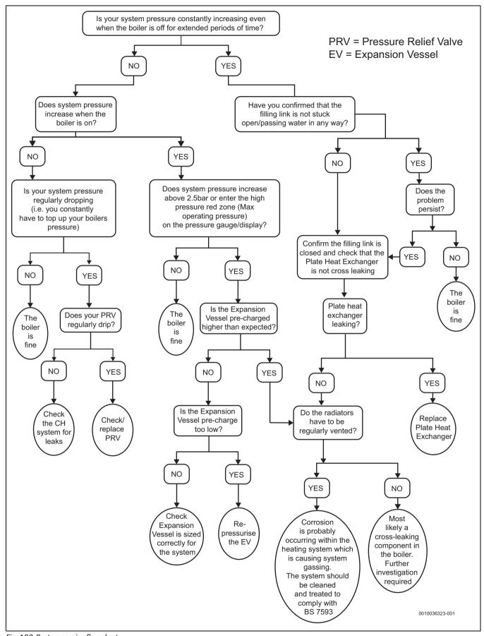
Fig. 103 System gassing flow chart
