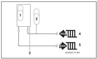
Fig. 4 Additional expansion vessel
