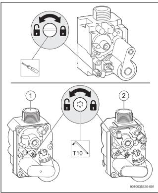
Fig. 62 Checking the gas supply pressure (above: SIT valve, below: Honeywell valves)
