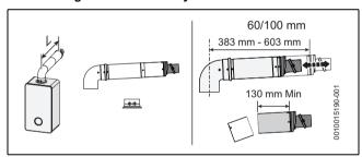
Fig. 14 Horizontal flue option
