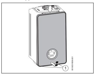
Fig. 68 Fitting the front casing
