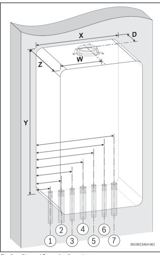
Fig. 2 Pipe and flue outlet dimensions
