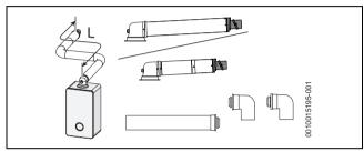
Fig. 19 Horizontal flue option
