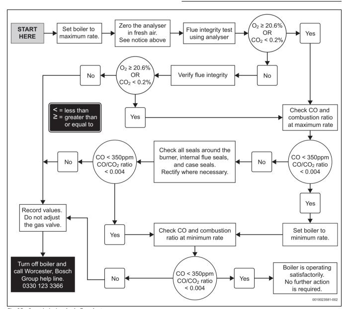
Fig. 65 Commissioning checks flow chart
