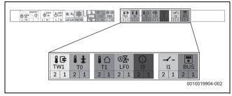
Fig. 59 Low voltage (signal cables) terminal strip
