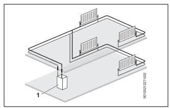
Fig. 6 Single central heating circuit example
