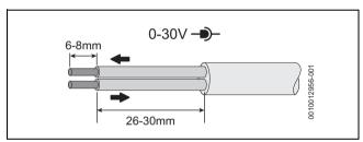
Fig. 54 Low voltage (signal cables) preparation
