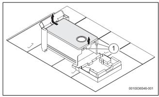
Fig. 42 Removing the front casing
