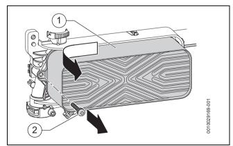
Fig. 95 Removing the plate heat exchanger
