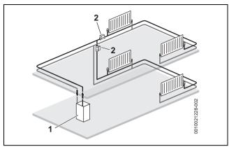
Fig. 7 Separated heating zones
