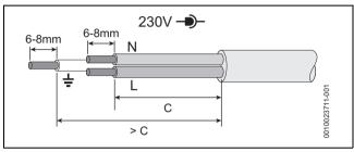
Fig. 53 Power supply (power cables) preparation
