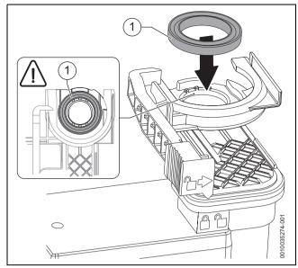
Fig. 80 Replacing the gasket
