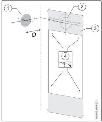
Fig. 43 Wall mounting template
