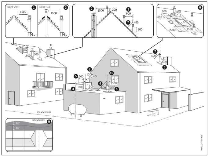
Fig. 30 Vertical flue terminal positions
