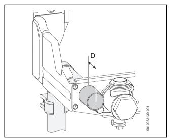
Fig. 45 Condensate drain pipework detail
