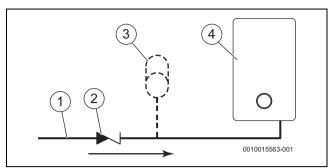
Fig. 9 Mini expansion vessel location
