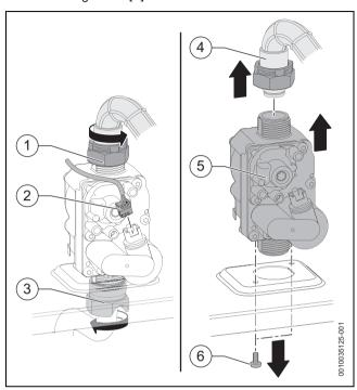
Fig. 94 Removing the gas valve
