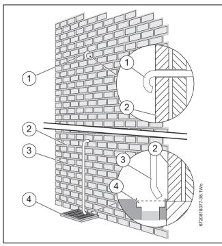
Fig. 41 Pressure relief pipework
