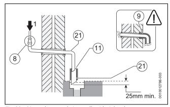
Fig. 38 Disposal to open drain or gully with air break
