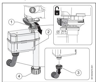
Fig. 79 Removing the siphon
