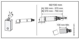
Fig. 15 Horizontal flue option
