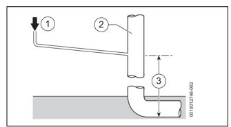
Fig. 33 Disposal to soil vent stack
