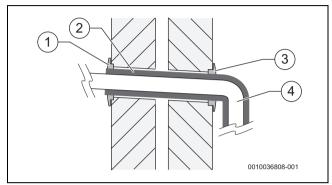
Fig. 40 Through the wall lagging example
