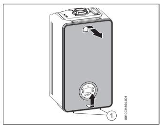
Fig. 84 Removing the front casing
