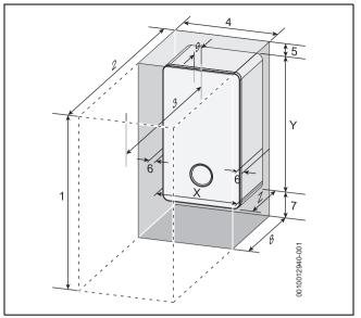
Fig. 11 Appliance minimum clearances
