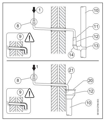
Fig. 37 Disposal into rain water down pipe
