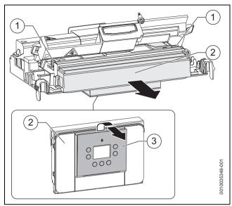
Fig. 102 Control unit removal
