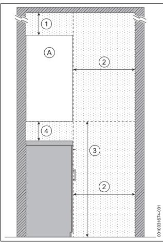
Fig. 12 Reduced front maintenance clearances - Side view
