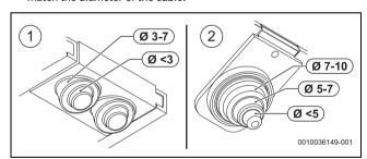
Fig. 56 Adapting the grommets to the cable diameter
