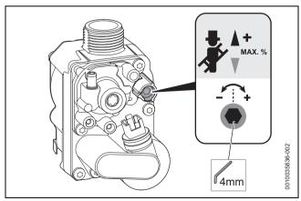
Fig. 83 Setting the CO<sub>2</sub> content
