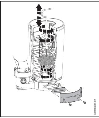
Fig. 76 Cleaning the heat exchanger
