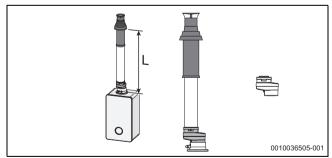
Fig. 27 SimpleSwitch flue adaptor
