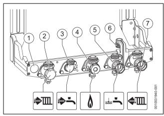
Fig. 44 Connections on the gas and water side
