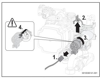
Fig. 89 Detaching the motor from the 3-way valve (variant without screws)
