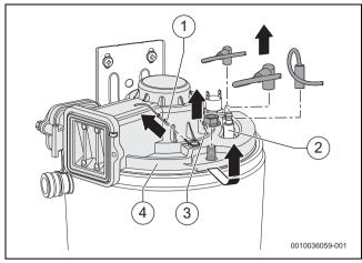
Fig. 72 Remove the burner cover
