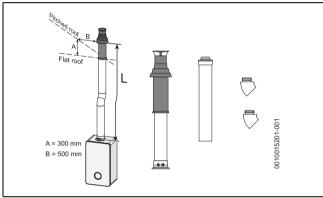
Fig. 26 Vertical flue option
