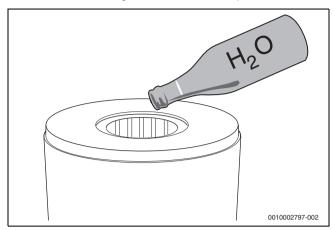
Fig. 77 Rinse the heat exchanger with water Refer to figure 78.
