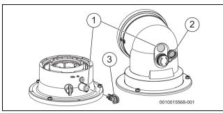
Fig. 66 Flue integrity check test point
