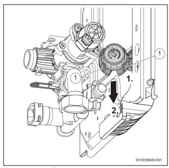
Fig. 100 Front view of pressure gauge
