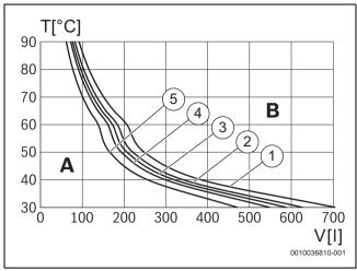
Fig. 5 Curves for the expansion vessel
