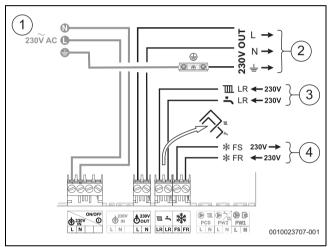
Fig. 60 External controls connections example
