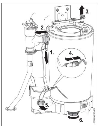
Fig. 85 Separating components from the heat exchanger assembly Removing the heat exchanger assembly Refer to figure 86.
