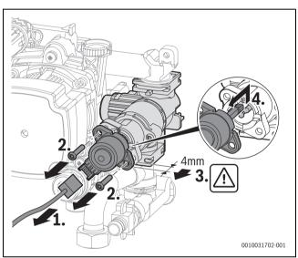
Fig. 91 Detaching the motor from the 3-way valve (variant with screws) Installing the motor.
