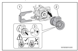
Fig. 88 Checking the flow turbine operation
