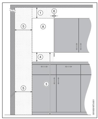
Fig. 13 Reduced front maintenance clearances - Front view
