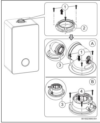
Fig. 52 Flue turret/adaptor connection
