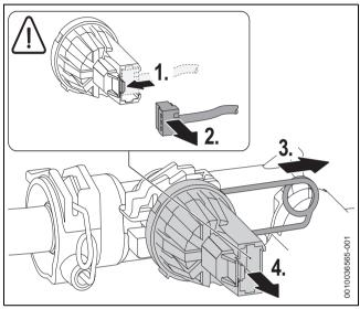
Fig. 98 Pressure sensor removal
