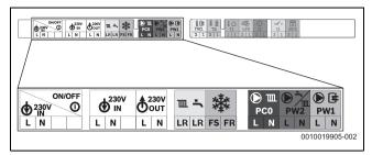
Fig. 57 Power supply (power cables) terminal strip
