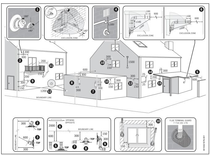
Fig. 32 Plume re-direct and plume management terminal positions
