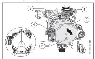
Fig. 93 Removing the pump
