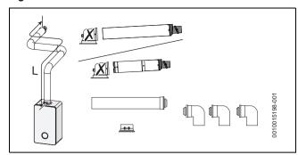
Fig. 22 Horizontal flue option
