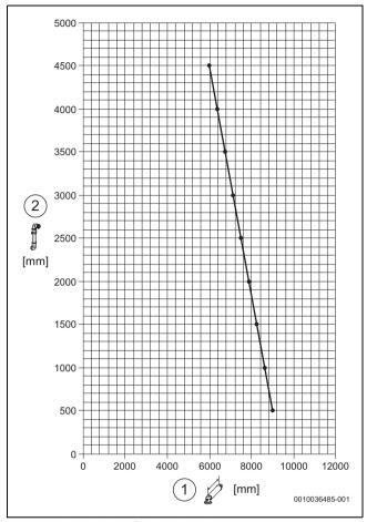
Fig. 28 Plume length to flue length graph
