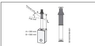
Fig. 24 Vertical flue option
