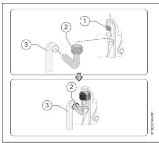
Fig. 46 PRV connection preparation
