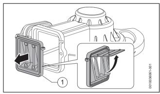
Fig. 73 Non-return valve (bearing plate) in the mixing unit Refer to figure 74.
