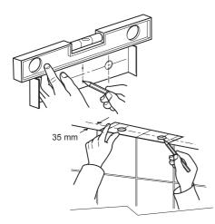
3. For solid walls drill the holes for the backplate with a 6 mm drill and insert the wall plugs.
