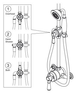
The diverter lever operates as shown above:
