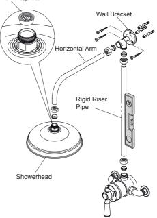
14.Temporarily fit the rigid riser pipe and wall bracket to the shower control outlet and mark the position of the wall bracket. Use a spirit level to ensure the pipe is vertical. Drill the holes and insert the wall plugs.
