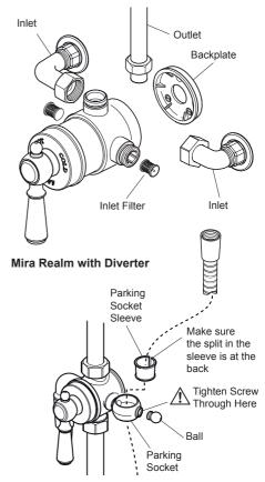
After a period of use the friction device on the parking socket may become loose, this can be tightened as follows:
