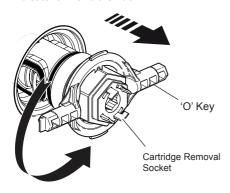
5. Fit the 'O' Key and cartridge removal socket (supplied) onto the cartridge nut and turn anticlockwise. Unscrew fully and pull the cartridge from the mixer body.
