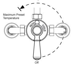
The Mira Realm thermostatic mixer is a thermostatic shower control with a single control lever for on/off and temperature control.
