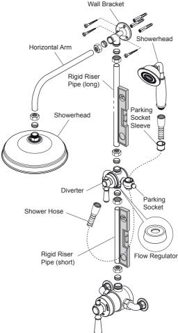
Temporarily fit the rigid riser pipe (short), diverter, rigid riser pipe (long) and wall bracket to the shower control outlet and mark the position of the wall bracket. Use a spirit level to ensure the pipes are vertical. Drill the holes and insert the wall plugs.
