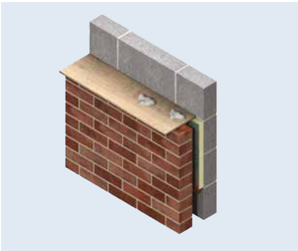
Figure 7 – Use of a Cavity Board to Protect the Cavity and Insulation Board Top Edge
