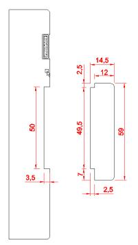
The tongued in stop and grooved frame linings are to comply with the material and dimensional requirements stated within the table in section 3.
