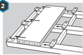
Place the first piece of decking on the timber frame with the decking running perpendicular to the joists. The first piece of deck may be secured with starter clips. **Do not** screw or nail through HD Deck® XS, use one Universal Clip and screw on every joist.
