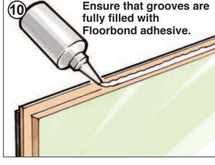
10 Ensure that grooves are fully filled with Floorbond adhesive.
