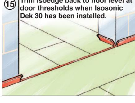
15 Trim Isoedge back to floor level at door thresholds when Isosonic Dek 30 has been installed.
