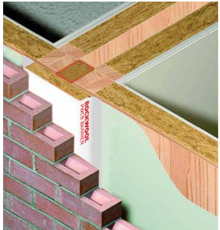
Figure 2 PWCB Cavity Barriers installed at separating wall position
