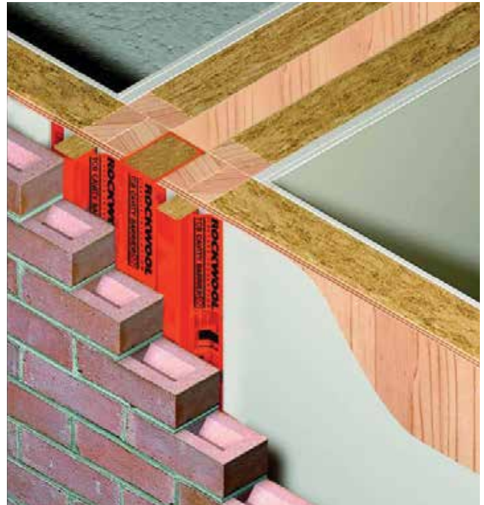
Figure 1 TCB Cavity Barrier installed at separating wall position
