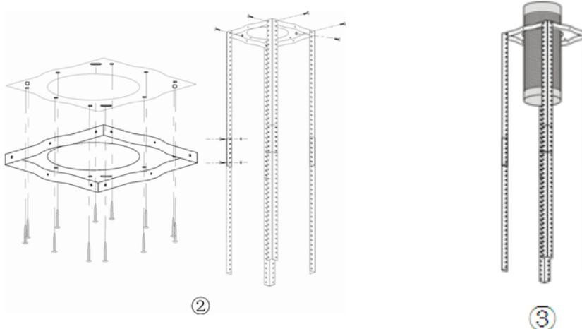
6. 4pcs ST4\*8 big flat screws will be used to connect the inside chimney into the hanging board, then put on the outside chimney, two hooks will be used to put up the outside chimney in order to the next installation, see pic 4.
