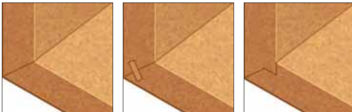
Mitre joints between Caberwood MDF panels
