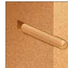
Dowel with 0.1mm all round clearance preferred
